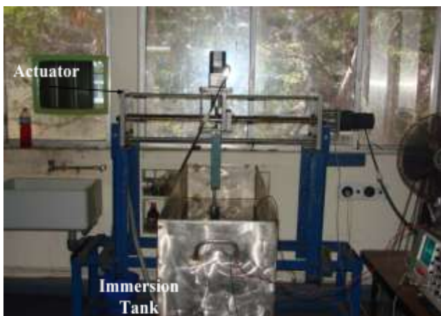
Figure 1: Immersion Tank with the Actuator (Courtesy: IGCAR, Kalpakkam)
