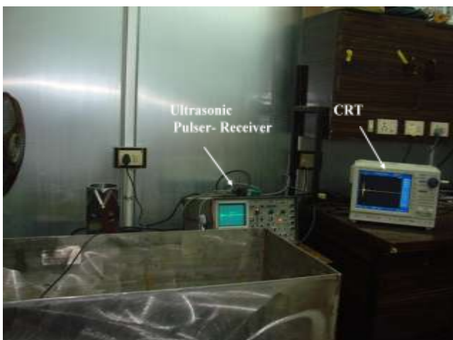
Figure 2: Recording and Display system (Courtesy: IGCAR, Kalpakkam) The transducer probe is also kept immersed in the water but at a certain height from the object, such that the object is in the far field of the transducer. The test object is the hexcan which is
