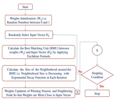
Figure 2 Flowchart of SOM Network Process [20].
