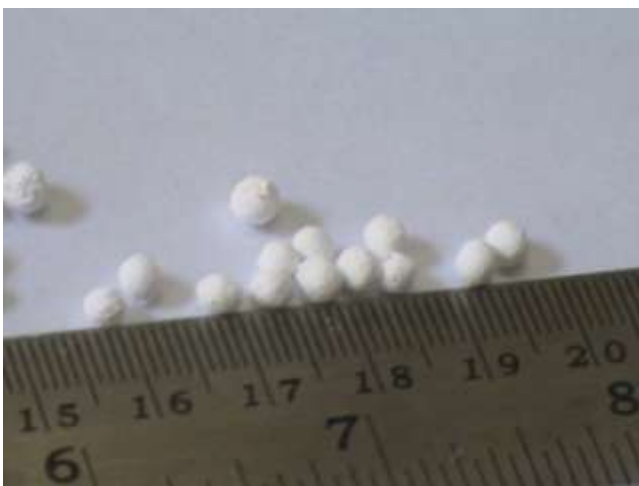
Fig.3 Calcined Lithium titanate pebbles of dia 3 mm (approx)
