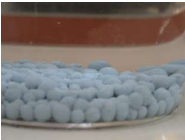
Fig.2 – Photograph of lithium metatitanate pebbles prepared by sol gel route followed by spherodization
