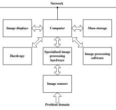
Figure: Digital Image Processing Components
