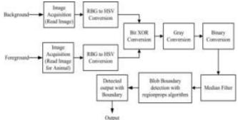
Figure 3.1: Block Diagram of animal detection using background subtraction
