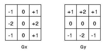
Figure 4.6: Sobel convolution kernels
