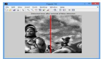
Figure 5.8: Detected scratch line after removal of false detection.
