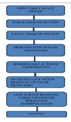
Figure 4.2: Proposed process flow of detection and removal of line scratches from video frame.
