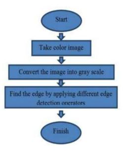
Figure 4.5: Flow chart for edge detection
