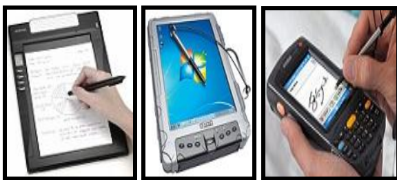
Figure:4 Devices to Capture Online handwriting; (a) Digimemo; (b) Tablet PC; (c) PDA
