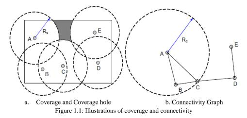
Figure 1.1(a) demonstrates a coverage illustration where the detecting angle of a sensor hub is displayed as a twofold circle. Each point inside the detecting range Rs of a sensor hub is thought to be secured by the hub. The union of the considerable number of circles structures the aggregate coverage of the network. The locale of interest is encased by a rectangle in the Figure. The shadowed locale is not secured by any sensor hub and in this manner thought to be a coverage opening.
