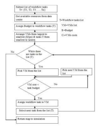
Figure 3.1 Basic Min-Min Budget Constrained Workflow Scheduling Algorithm
