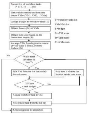
Figure 3.2 Score Based Min-Min budget Constrained Workflow Scheduling Algorithm
