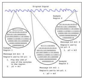
Fig 8:- Parity Coding Procedure.
