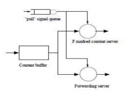
Fig. 3. Queue Model of Source Server
