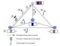
Fig. 1.Queue-based P2P system with four nodes.
