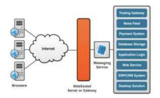
Fig1.Architecure of websocket protocol server.
