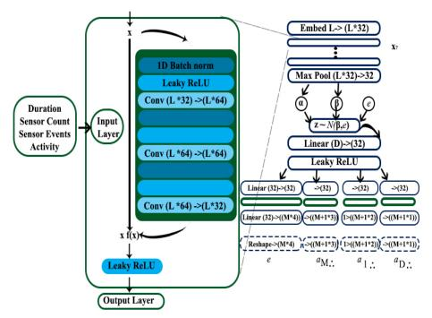
Figure-2 Overall architecture of Auto Encoder with Hidden Markov Model (AE-HMM)
