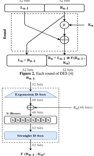
Figure 3. The working of DES F Function [5]
