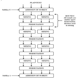
Figure 9. First Four Round Operations of the Threefish-256 Cipher [14]
