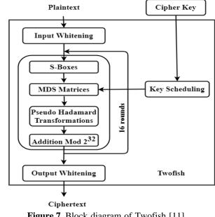
Figure 7. Block diagram of Twofish [11]
