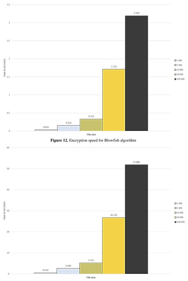
Figure 13. Encryption speed for Twofish algorithm
