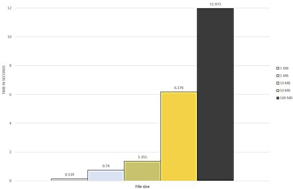
Figure 11. Encryption speed for 3DES algorithm
