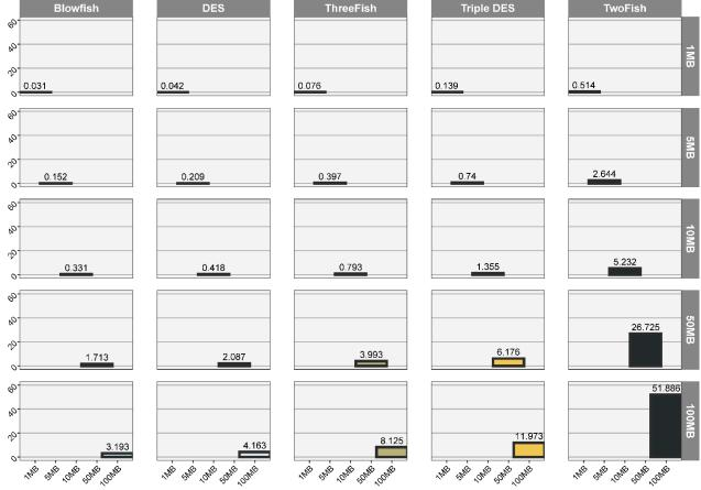
Figure 15. Comparison of encryption speed for DES, 3DES, Blowfish, Twofish, and Threefish.
