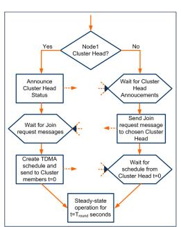
Figure 3. Set-up phase flowchart.
