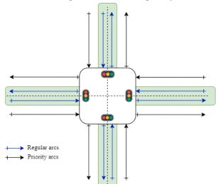
Figure 2. Intersection of two ordinary roads and two priority
