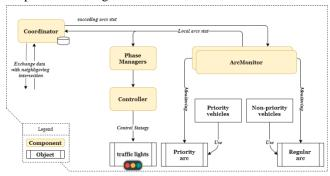
Figure 3. The components of the generic TSCS
