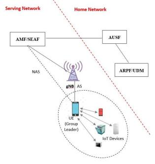
Figure 3: Security architecture of 5G-IoT
