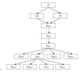
Figure 5: Keys generated during 3GPP 5G-AKA
