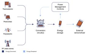
Figure 1. Energy harvesting flow of IoT devices
