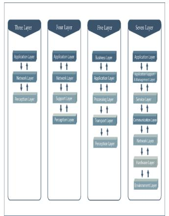
Figure1. The Layered Architectures of IoT
