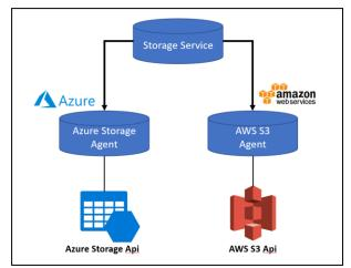
Figure 5. SBS approach applied for two public cloud interoperability (Azure, AWS)
