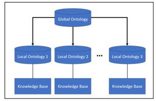
Figure 3. Generic architecture for Hybrid Ontologies.
