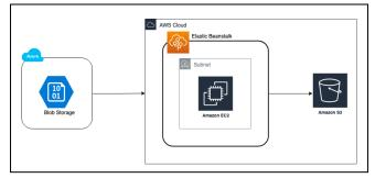
Figure 13. A pictorial representation of a Azure Blob Storage to AWS S3 migration architecture [32]
