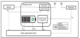
Figure 1. The recovery-aware battery powered study system
