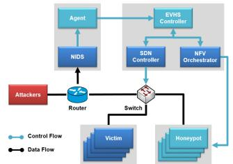
Figure 3. System architecture.
