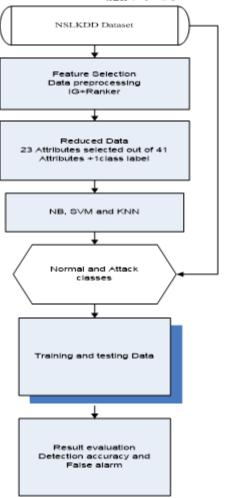
**Figure 1.** Block diagram of proposed IG+R-NB, IG+R-SVM and IG+R-KNN
