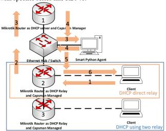
Figure 6. Smart Agent and DHCP relay in default Mikrotik Scenario with "Capsman" protocol
