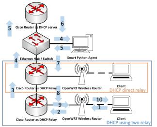
Figure 3. Smart Agent and DHCP relay using Smart Agent Cisco Scenario with two relay
