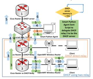
Figure 4. Smart Agent and DHCP relay using Smart Agent Cisco Scenario when DHCP relay take over the DHCP server duty
