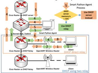
Figure 2. Smart Agent and DHCP relay using Smart Agent Cisco Scenario
