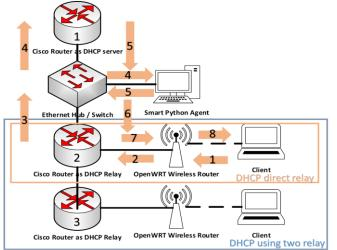
Figure 1. Smart Agent and DHCP relay in default Cisco Scenario
