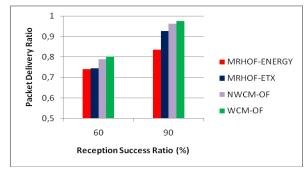
Figure 5. Performances in term of packet delivery ratio for 40 nodes.
