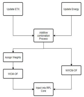
Figure 3. Proposed objective functions injected into RPL core
