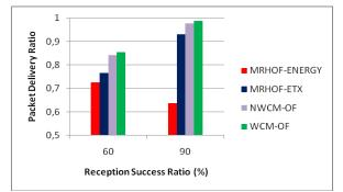
Figure 4. Performances in term of packet delivery ratio for 20 nodes.
