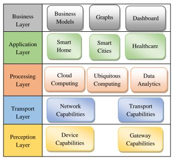
Figure 4. Five-Layer IoT Architecture
