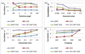
Figure 6. Behavior of the correlation coefficient between the original watermark and extracted watermark for the different attacks. (a) Rotation. (b) Gaussian noise. (c) Resizing. (d) Cropping.
