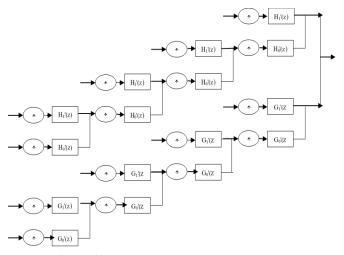
Figure 1. Dual-Tree discrete CWT decomposition
