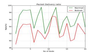
Figure 9. Packet delivery ratio during normal and attack period
