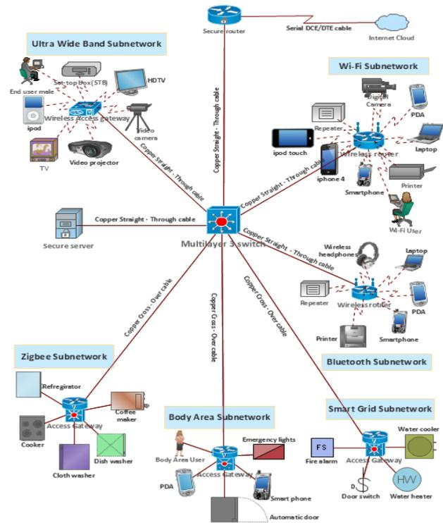
**Figure 1.** A typical IHN system architecture proposed in [2,3]
