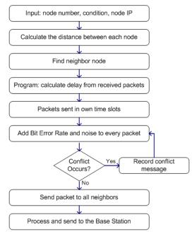
Figure 3. Flow diagram of SRA.
