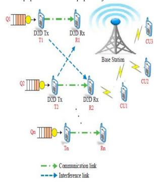
**Figure 2.** Interference in Device to Device communication For downlink transmissions, the D2D receivers are synchronized with their closest D2D transmitters [13]. D2D transmitters use path-loss inversion power control techniques to transmit data in a cell. The devices are classified into primary and secondary nodes based on the distance and the algorithm derives the required transmit power for communication.
