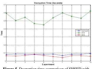
Figure 5. Decryption time comparison of SHSED with AES and DES
