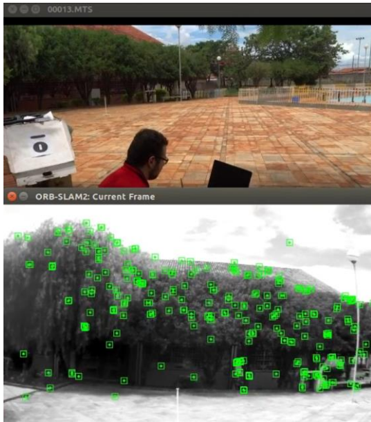
Figure 2. The first image shows the outdoor scenario of the experiment captured by a video camera. Second image shows the front image of AR.Drone 2.0 using ORB SLAM2 package.
