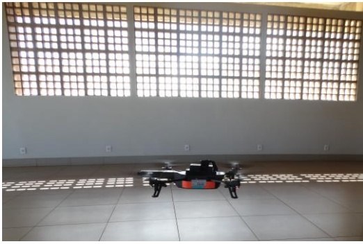
Figure 4. Parrot AR.Drone 2.0 robotic platform used in the experiments.
