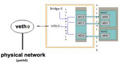
Figure 6. Network-Bridge and VIF-Bridge connectivity in Xen
