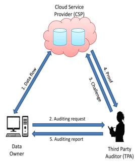
Figure 2. Architecture of system model
