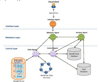
Figure 8. Architecture of the proposed multi-agent system model
