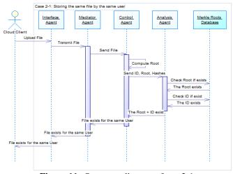
Figure 11. Sequence diagram of case2-1
