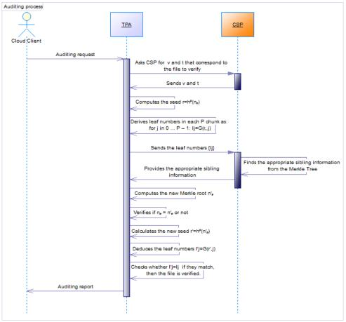
Figure 14. Sequence diagram for auditing a file
