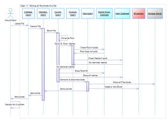
Figure 9. Sequence diagram of case1-1
