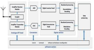
Figure 6. Synoptic diagram of SDR card
