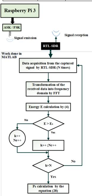
Figure 17. Chart of the energy detection operation
