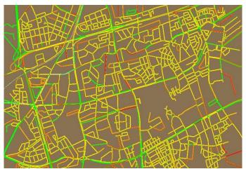
Figure 13. The traffic  $CO_2$  emissions in the last scenario.
