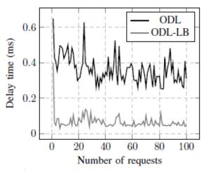
Figure 4. Delay time for 100 ping requests between h1 and h12.
