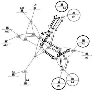
Figure 7. Network load balancing.
