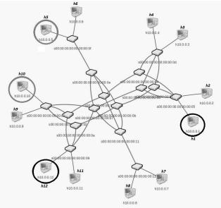
Figure 8. Network from Floodlight API Web.
