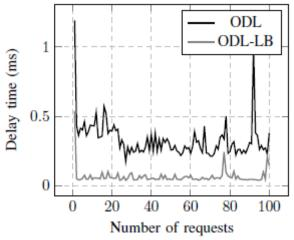
Figure 5. Delay time for 100 ping requests between h3 and h8.
