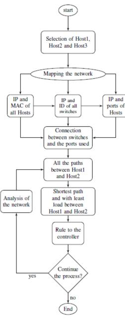
Figure 2. Flow diagram of the proposed load balancing algorithm.
