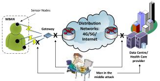
**Figure 1.** Possible attack points for unsecure ECG signals subjected to man in the middle attack.
