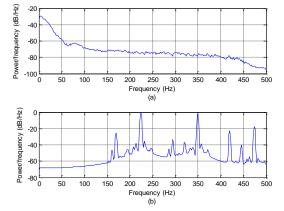
**Figure 5**. Power spectral density representation of normal ECG signal: (a) original ECG signal, (b) anonymised ECG signal for P = 1,024.
