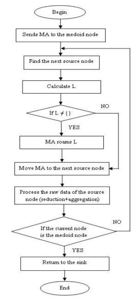
Figure 7. Flowchart of the communication process of mobile agents
