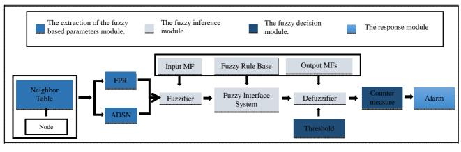
Figure 2. The normal proposed system in detail
