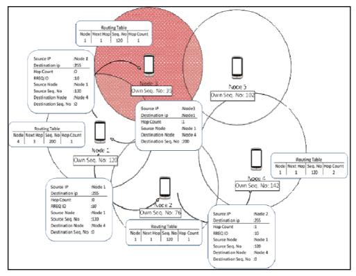
Figure 1. The black hole attack process
