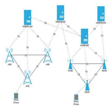
Figure 1. Integration of Femtocell in LTE network i.e. Two tier network.
