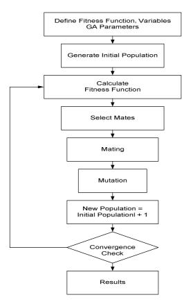
Figure 2. Stages of the GA Process
