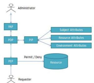
Figure 3. The XACML Structure in Data-Centric Level Access Control
