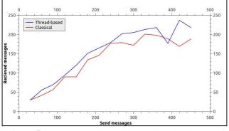
Figure 5. Comparison of the amount of received messages on 30 cycles – Classical Vs Thread-based
