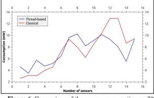
Figure 6. Comparison of the energy consumption on 30 cycles – Classical Vs Thread-based
