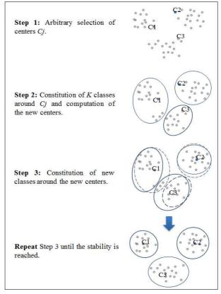
Figure 2.Network partitioning using the k-means method
