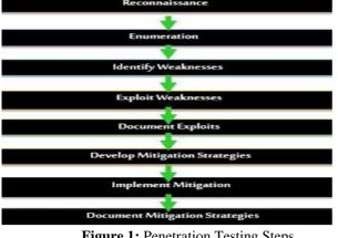
Figure 1: Penetration Testing Steps.
