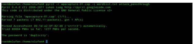
Figure 8: Ouput of the "pyrit -r wpacapture-01.cap -I wordlist.txt attack\_passthrough" command.
