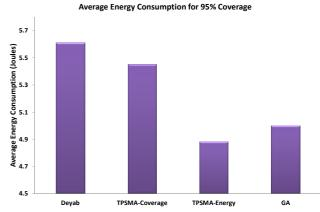
Figure 6. Average energy consumed by each sensor node for minimum of 95% coverage
