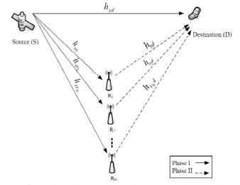
Figure 1. An integrated satellite-terrestrial cooperative system
