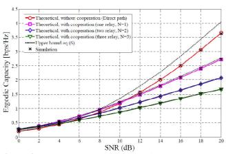
**Figure 3:** Ergodic capacity analysis of the multiple relay integrated satellite-terrestrial cooperative system, when the direct channel  $S \rightarrow D$  experience deep shadowing,  $m_0 = 2.56$ , while the  $S \rightarrow R_i$  channel have LOS,  $m_0 = 26$  and  $R_i \rightarrow D$  channel experience Nakagami-2 fading
