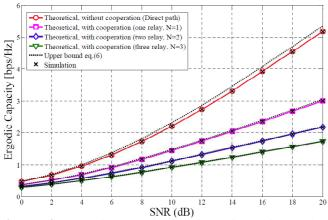
**Figure 4:** Ergodic capacity curves of multiple relay integrated satellite-terrestrial cooperative system, when the satellite channels,  $S \rightarrow D$  and  $S \rightarrow R_i$  experience moderate and light shadowing respectively where  $R_i \rightarrow D$  link experience Nakagami-*m* fading at m = 1.
