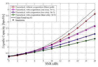
**Figure 2**: Ergodic capacity analysis of the multiple relay integrated satellite-terrestrial cooperative system, the direct channel  $S \rightarrow D$  experience deep shadowing,  $m_0 = 2.56$ , where the  $S \rightarrow R_i$  channel have LOS,  $m_0 = 26$  and the  $R_i \rightarrow D$  channel experience Nakagami- *m* fading at m = 1
