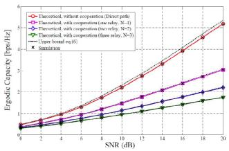
**Figure 5:** Ergodic capacity curves of multiple relay integrated satellite-terrestrial cooperative system, when the satellite channels,  $S \rightarrow D$  and  $S \rightarrow R_i$  experience moderate and light shadowing respectively where the  $R_i \rightarrow D$  link experience Nakagami-2 fading.
