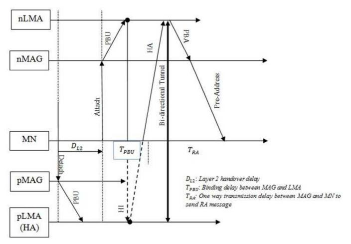
Figure 9. Novel Inter-domain PMIPv6 Handover Procedure and timing diagram
