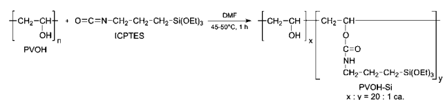
Scheme 1 Reaction scheme of the preparation of triethoxysilane functionalized polyvinyl alcohol [PVOH-Si].
