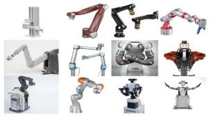
Figure 5: Various off-the-shelf collaborative robots
